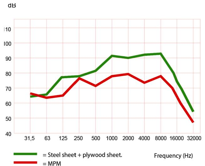
Fig. 1. Shows the sound pressure level when working on a chute produced of MPM in relation to a chute produced of a steel sheet + a plywood sheet. By using MPM the sound pressure level is reduced with approx. 14dB.
